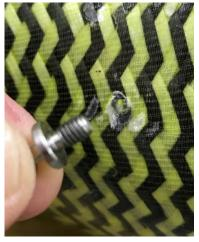
Apply thread locker to the stud threads, and screw the stud into the hole and into the Star Nut.
