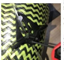
NOTE: Do not tighten set screw completely in case length needs to be adjusted!
